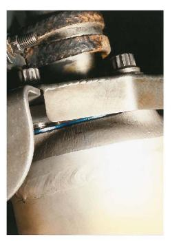
Figure 5: CF6 Gap at Leaking Flange
