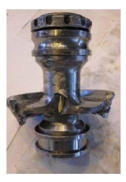
Figure 4: GE90 Transfer Gearbox Pinion Gear
