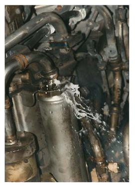
Figure 6: CF6 Wet Motor Leak Test
