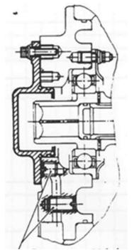
Figure 7: CFM56 Hand Cranking Pad Schematic
